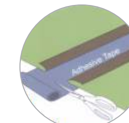
Fold the trimmed edges; put the adhesive tape below the edges
